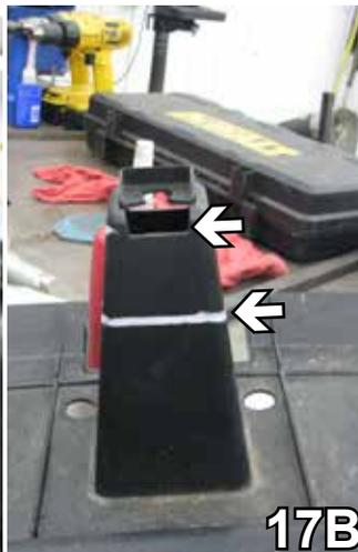
17. On the center extension, measure down 3/4", using the utility knife cut around the top, 2 1/2" down and straight across.
