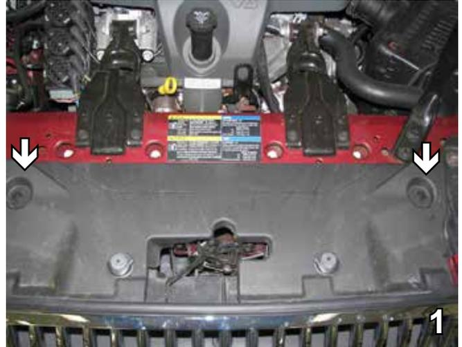
1. Remove two push pins from the top of the plastic cover. Set cover and push pins aside to be reinstalled later.
