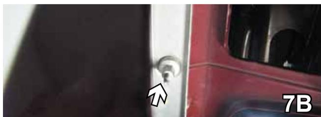
7. Just forward of the front tire push the wheel well cover aside, using the 10mm socket, loosen two metric bolts. Do this to both sides of the vehicle. Pull fascia forward to remove. Set bolts and fascia aside carefully to be reinstalled later.
