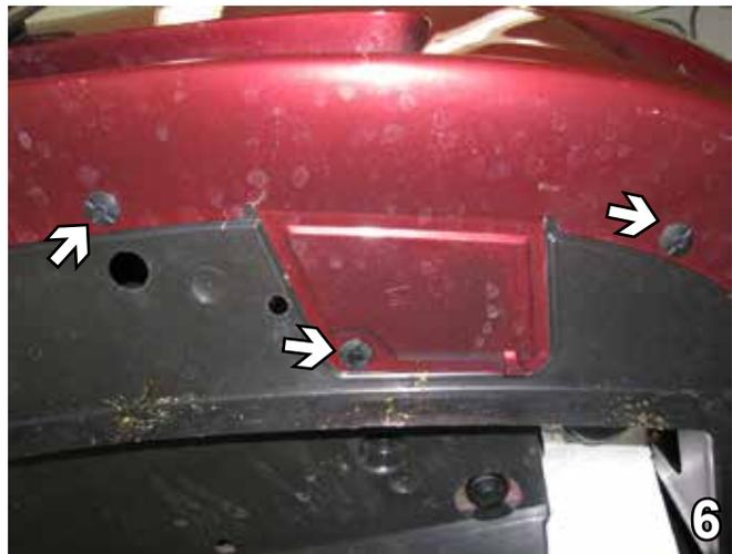
6. Remove three push pins from bottom corner of fascia. Do this to both sides of the vehicle. Set push pins aside to be reinstalled later.
