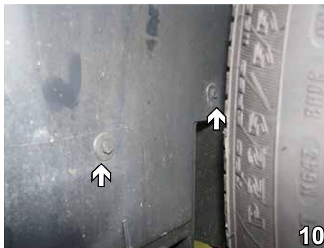
10. Just forward of the front tire, on the wheel well using the 7mm socket, remove two bolts. Pull forward on the center extension to remove the belly pan. Set belly pan and bolts aside to be reinstalled later.
