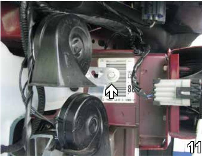
11. On the passenger side, using the 10mm socket, remove one metric bolt from the horn bracket. Set the horn and bolt aside to be reinstalled later.
