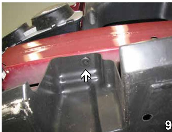
9. Remove two push pins from the belly pan extensions one on each side. Set push pins aside to be reinstalled later.
