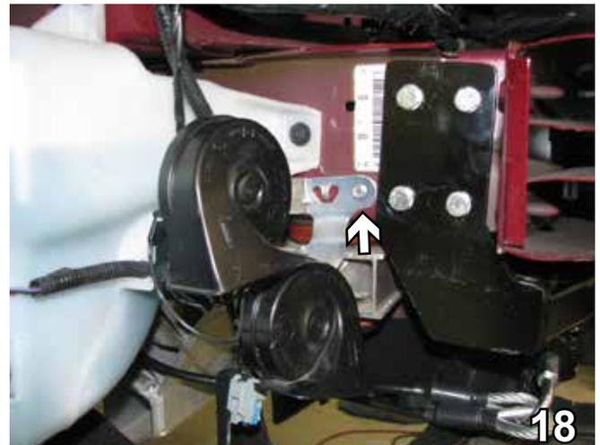
18. Remount the horn bracket, using a self tapping screw.
