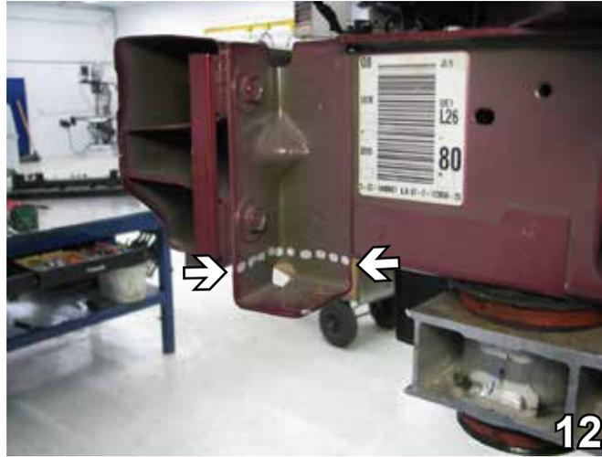
12. Using the reciprocating saw, mark and cut the bottom of the bumper bracket so that it is flush with the bottom of the frame rail. Do this to both sides of the vehicle.
