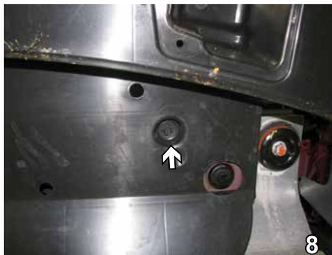
8. Using the 10mm socket, remove three metric bolts from across the bottom of the belly pan underneath the bumper. Set bolts aside to be reinstalled later.
