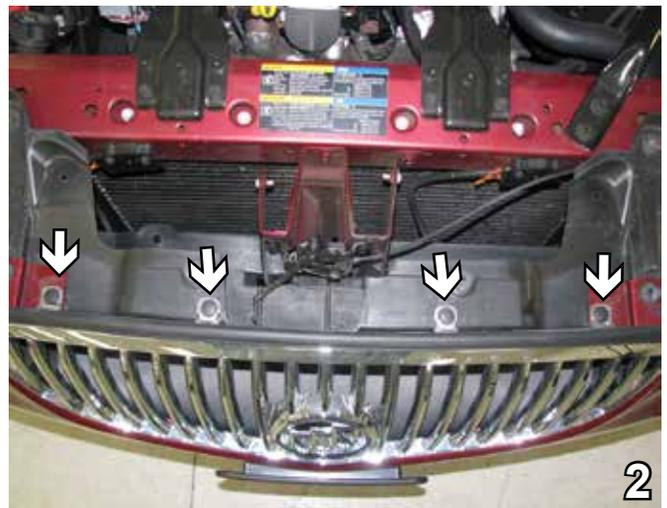
2. Remove four push pins from the top of the fascia. Set push pins aside to be reinstalled later.
